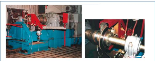
Fig.1. Disc brake - full view and detailed view
